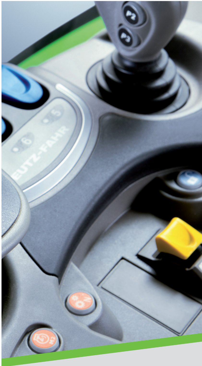
Three hydraulic valves are controlled via a simple joystick with integrated smart wheel.
