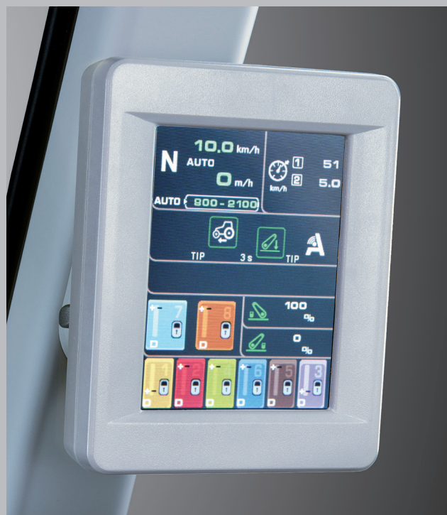
Three driving or work strategies can be selected. Manual, automatic and PTO. They are displayed in the WorkMonitor.
