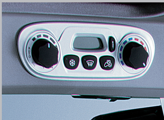
Pre-select temperature; the automatic controls precisely regulate the air flow.
