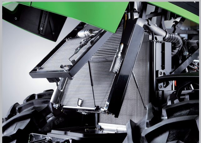
The radiator can be quickly unfolded and cleaned.
