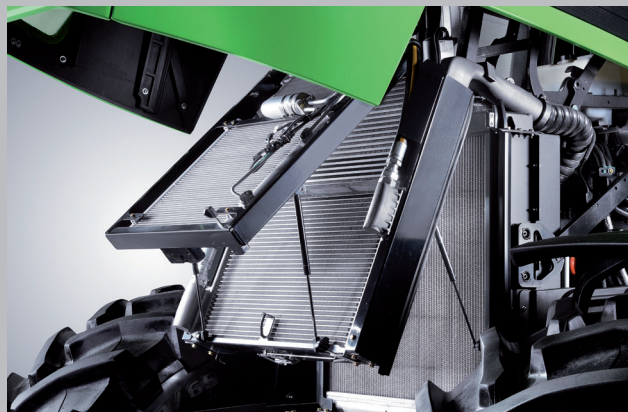
The compact cooling system enhances engine efficiency and is easy to maintain.
