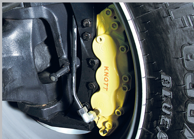
Dry disc brakes on the front axles for extra-safe braking effect (optional).
