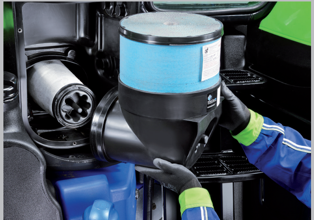
The engine air filter can be easily accessed and replaced.
