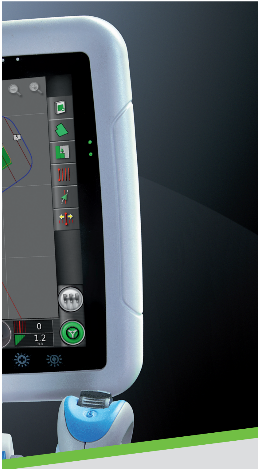
The Agrosky receiver. All satellite systems and correction signals can be received by a single device.
