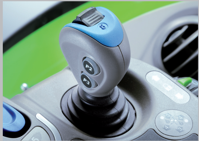
Three hydraulic valves are controlled via a simple joystick with integrated smart wheel.
