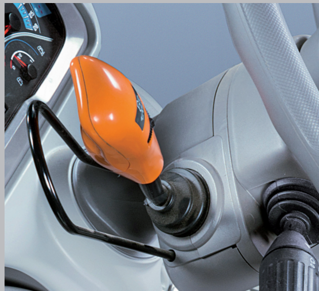
Standard: Power shuttle system. The shuttle sensitivity (hard – medium – soft) can be easily adjusted with the thumb.
