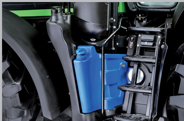
600 l diesel and 55 l AdBlue are sufficient for more than one day of hard work in the field. Optional: Fuel pre-heating for the best cold-start performance.
