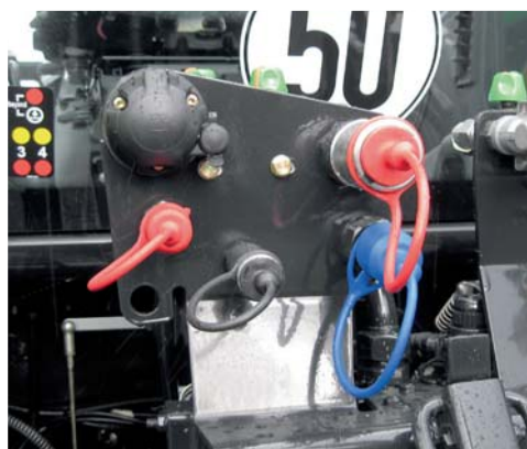
To order the Agrotion M can be fitted with Power-Beyond connectors for the direct connection of third-party devices.
